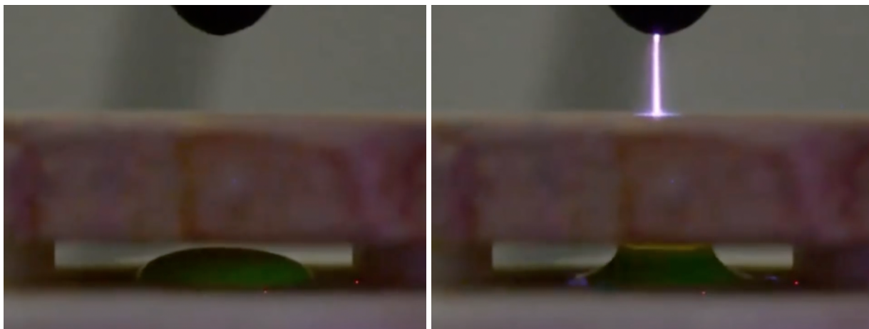
Figure 4: Direct current through sandstone (top), water with Pyranine, and quartz (bottom). The attractive force of the current pulls the water along the current against gravity, pushing up on the sandstone.
